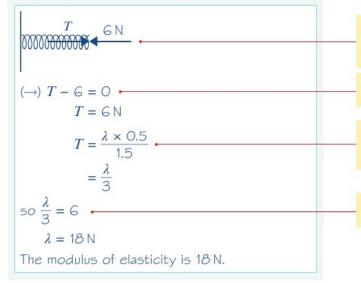
Draw a diagram showing the applied force 6 N and the thrust force T produced in the spring.
