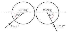
A small smooth sphere A of mass 1 kg collides with a small smooth sphere B of mass 2 kg. Just before the impact A is moving with a speed of  $4 \,\mathrm{m \, s^{-1}}$  in a direction at  $45^{\circ}$  to the line of centres and B is moving with speed  $3 \,\mathrm{m \, s^{-1}}$  at  $60^{\circ}$  to the line of centres, as shown in the diagram. The coefficient of restitution between the spheres is  $\frac{3}{4}$ . Find:
