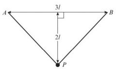
A light elastic string, of natural length 3*l* and modulus of elasticity  $\lambda$ , has ends attached to two points A and B where AB = 3l and AB is horizontal. A particle P of mass m is attached to the midpoint of the string. Given that P rests in equilibrium at a distance 2l below AB, as shown in the figure,
