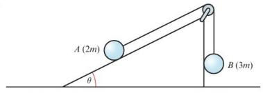
The diagram shows a particle A of mass 2m which can move on the rough surface of a plane inclined at an angle  $\theta$  to the horizontal, where  $\sin \theta = \frac{3}{5}$ . A second particle B of mass 3m hangs freely attached to a light inextensible string which passes over a smooth pulley.
