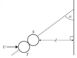
A small smooth uniform sphere S is at rest on a smooth horizontal floor at a distance d from a straight vertical wall. An identical sphere T is projected along the floor with speed U towards S and in
