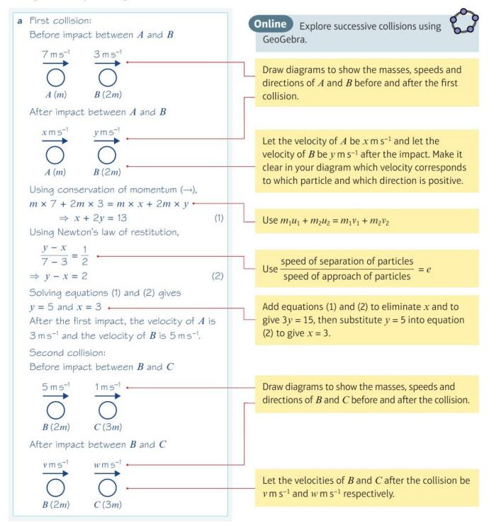
Using conservation of momentum  $(\rightarrow)$ ,  $2m \times 5 + 3m \times 1 = 2m \times v + 3m \times w$   $\Rightarrow 2v + 3w = 13$  (3)
