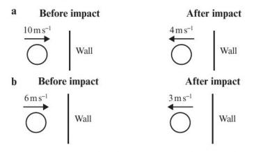
**2** A smooth sphere collides normally with a fixed vertical wall. The two diagrams show the speed and direction of motion of the sphere before and after the collision. The value of *e* is given in each case. Find the speed of the sphere after the collision in each case.
