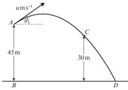
A particle P is projected from a point A with speed u m s<sup>-1</sup> at an angle of elevation  $\theta$ , where  $\cos \theta = \frac{4}{5}$ . The point B, on horizontal ground, is vertically below A and AB = 45 m. After projection, P moves freely under gravity, passing through a point C, 30 m above the horizontal ground, before striking the ground at the point D, as shown in the figure above.
