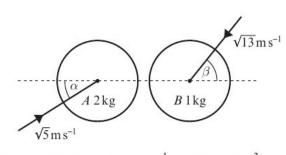
motion of A and an angle  $\beta$  with the direction of motion of B, where  $\tan \alpha = \frac{1}{2}$  and  $\tan \beta = \frac{3}{2}$ , as shown in the diagram above. The coefficient of restitution between A and B is  $\frac{1}{2}$ .
